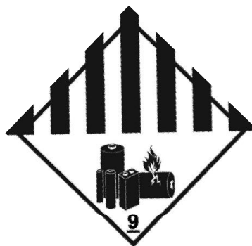
Figure 9-1: Class 9 Miscellaneous Dangerous Goods and UN Identification Label
