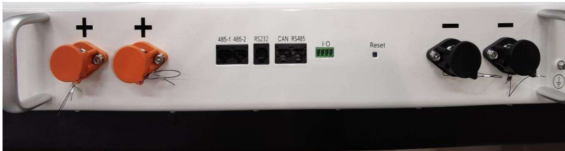
Figure 2: Powerline-5 pin-out image showing 485-1 & 485-2 ports:
