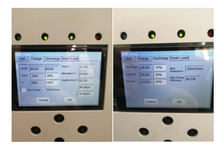
After setup, you can press 'Li-Batt info' to check battery Voltage/Current/Max Charge/Discharge current/SOC.
